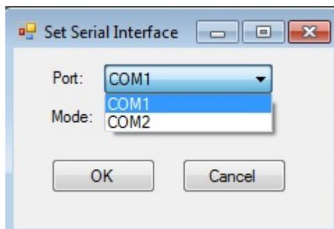
3. Select the serial interface mode for the port from the **Mode** dropdown box.
