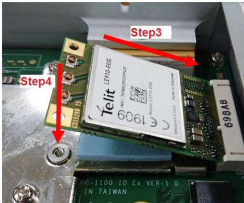
**STEP 5:** Secure the wireless module card with the 2 screws included in the package.
