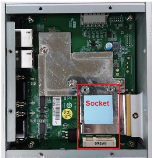
**STEP 3:** Insert the wireless module card at an angle.
